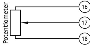
Resistance value is measured between **16** and **17** terminals.
